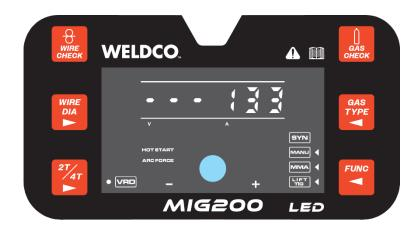
□ Ensure the main power switch (30) is in the OFF position. Plug the 10amp plug into the 10amp wall socket. Turn power to the ON position on both the wall socket and the power source. The front panel will illuminate, and the cooling fan will start.
